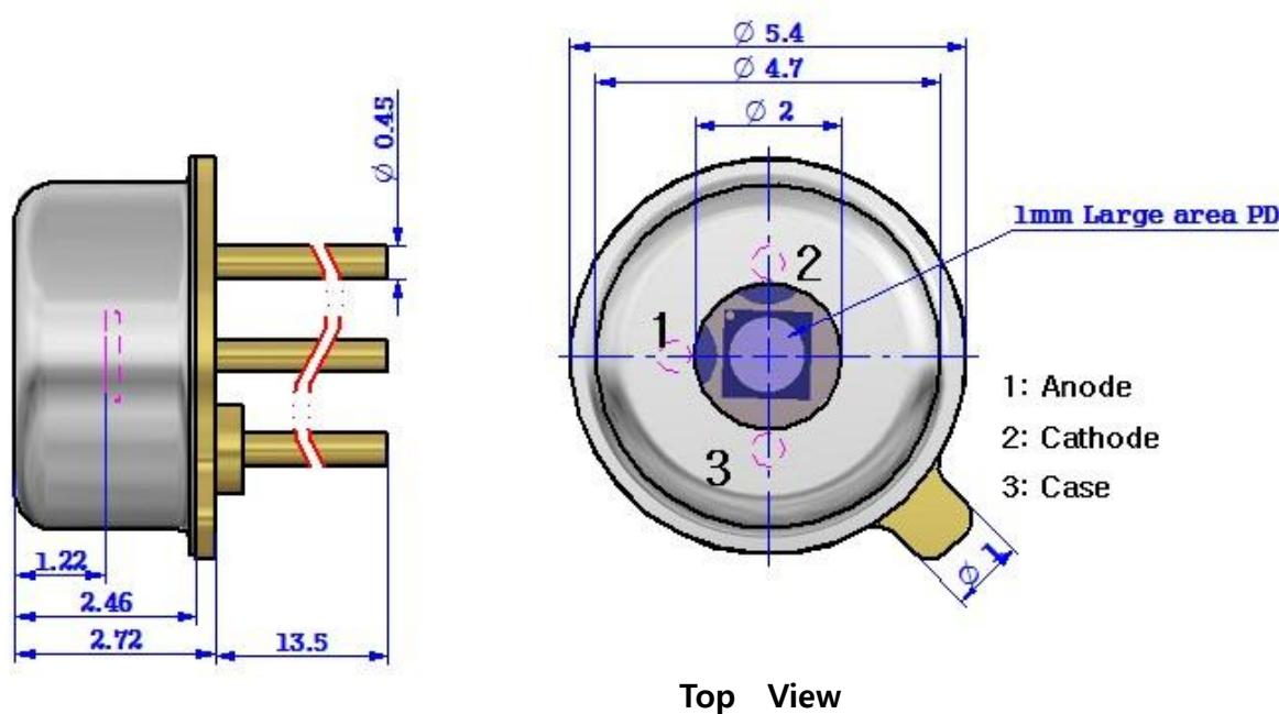
Figure 1. Dimensions Diagram
